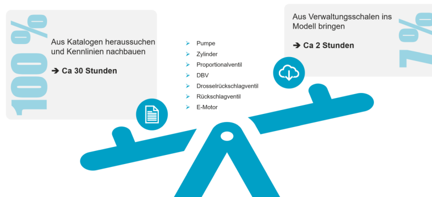
Figure 5.2. Time required for parameterization of components
