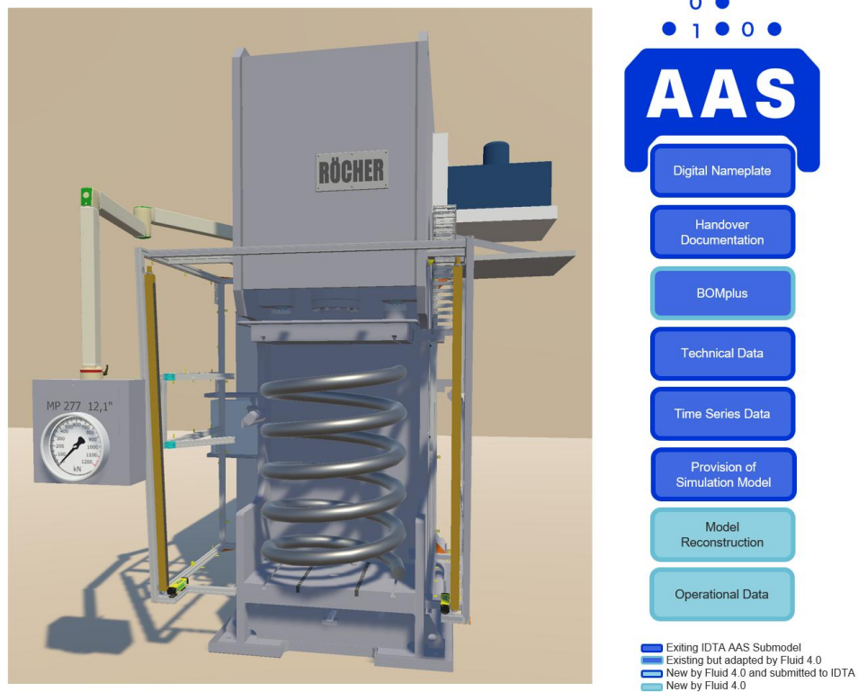
Figure 1.1. Fluid 4.0 example simulation of a hydraulic forming press
