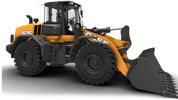
Figure 2.1. Wheel loader Case 821G
