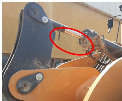
Figure 2.3. Detail of bucket cylinder with displacement sensor installed.
