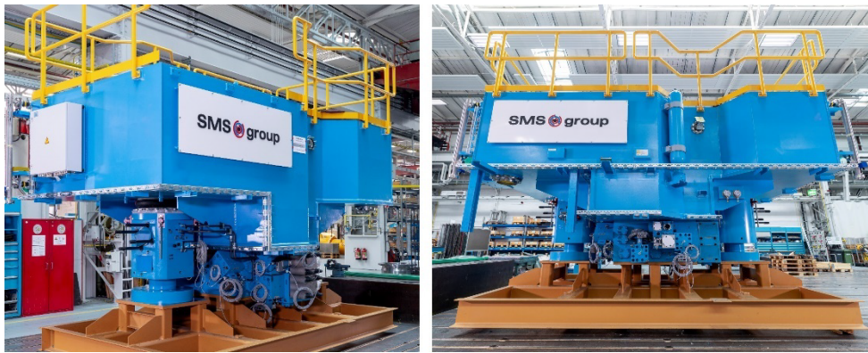
Figure 5.4. Integration of the forging manifold into the machine structure.
