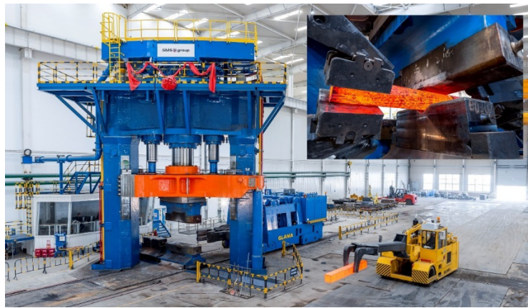
Figure 5.1. Exemplary open-die forging press.
