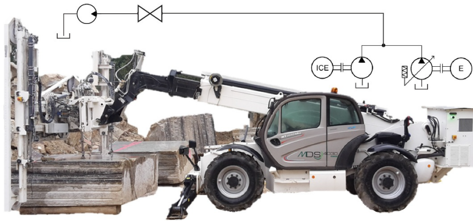
Figure 2 Hydraulic setup of the saw motor
