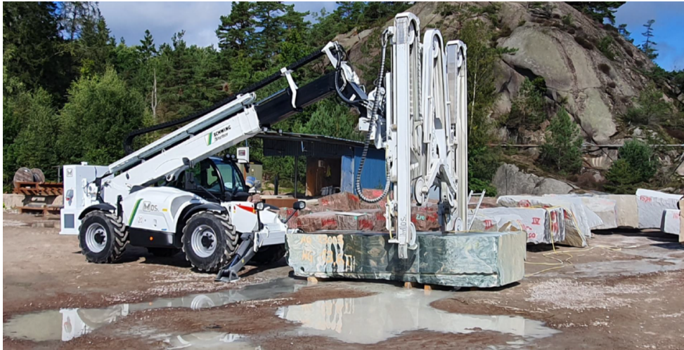
Figure 1 Wire saw attachment cutting, mounted on carrier vehicle including internal combustion engine and electric powerpack at the back
