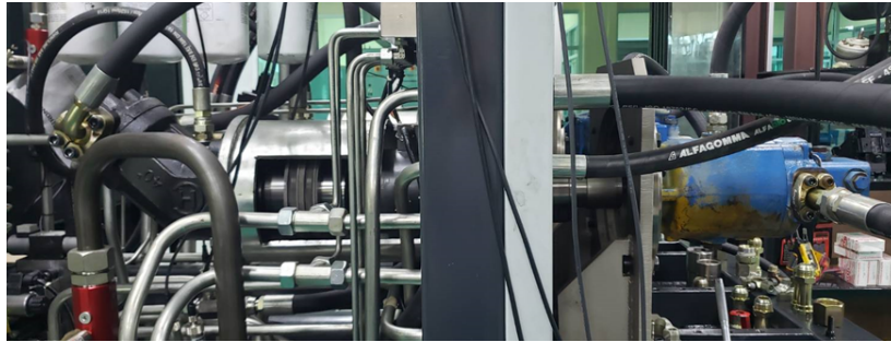
Figure 1. Cross-sectional view of the repaired hydraulic motor installed in the test rig and connected as a load motor.
