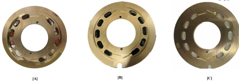
Figure 4.2. Wear observed on valve plate after experimental tests. [A]: Baseline design, [B]: Improved Port Block, [C]: Increased Interface Area
