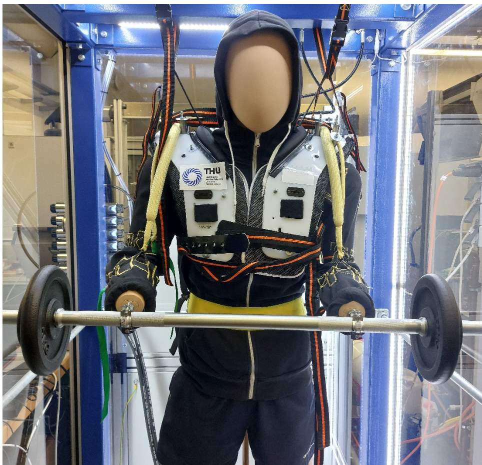
Figure 5.1 Exoskeleton test setup for power support for the upper body (here 20 kg)
