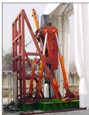
Figure 2: (left) test bench for hydraulic breakers; (right) impact absorbing base [4]. Text boxes were added by the authors.
