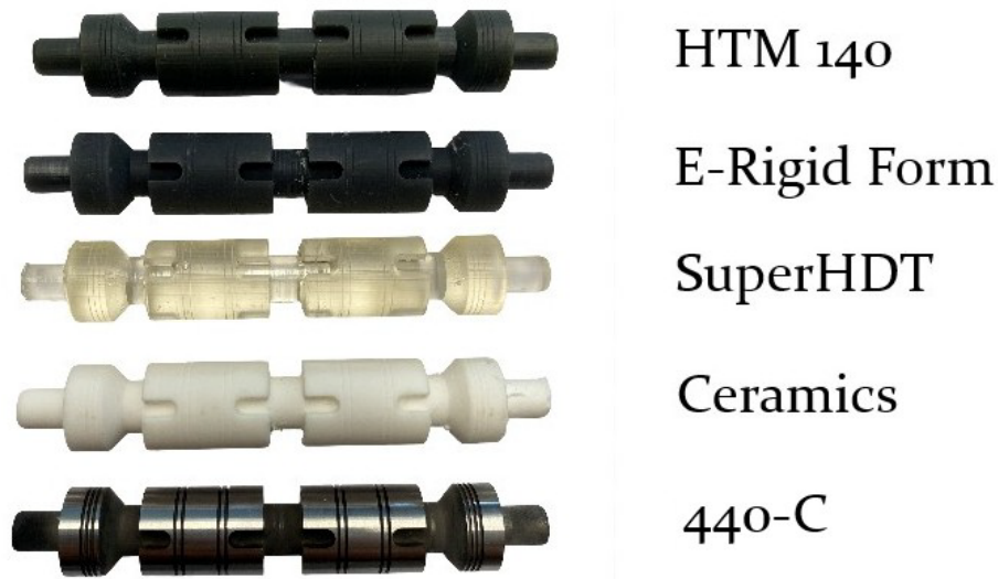
Figure 3: Spools made from alternative materials and standard spool made from AISI 440-C.
