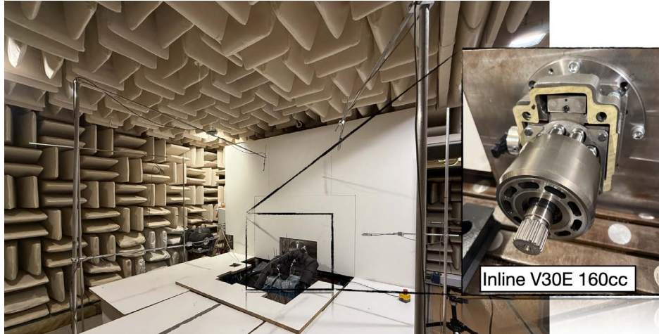
Figure 3.2. Test rig and 160cc test pump
